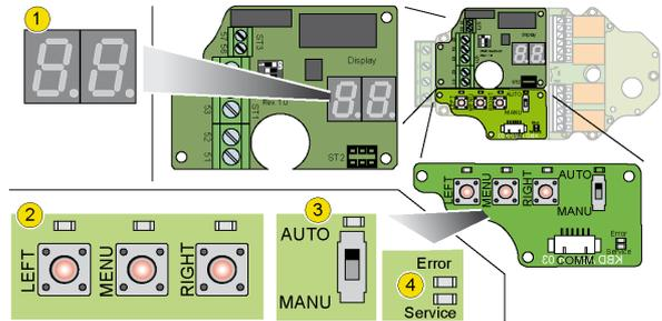
Two 7-segment displays (1) provide information on the controller status and the operating steps. The controller is configured and operated with the three keys (2) and the switch (3). The small LEDs above the buttons and the switch and the two LEDs (4) below the switch indicate various operating states and messages.
