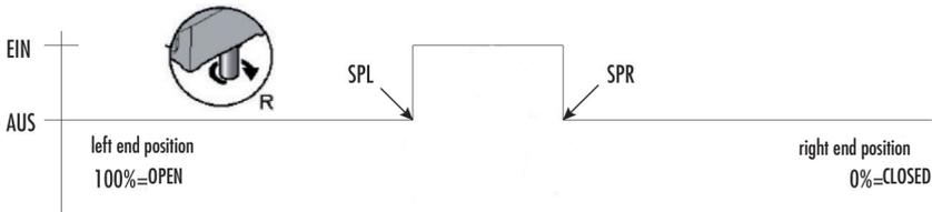
By defining and positioning of these two switching points different shift pattern can be freely defined.
