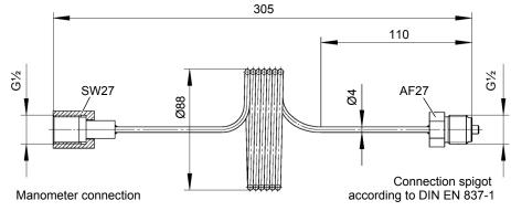
Fig. 7: Capillary throttle MZ400#
