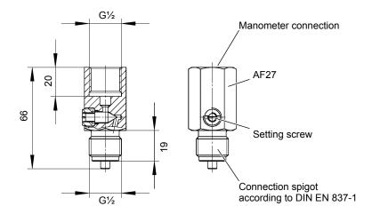
Fig. 8: Damping reactor MZ410#
