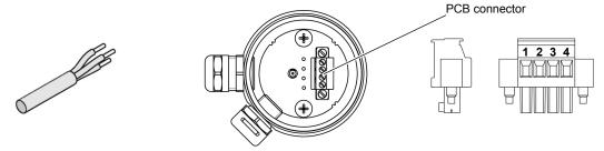
Fig. 14: Cable connection (field casing)
