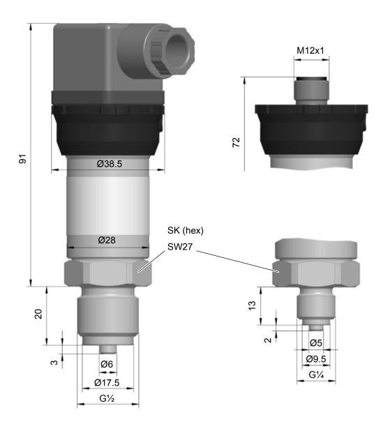
Fig. 15: Standard casing dimensional drawing
