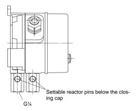
In the operational status, the reactor pins need to be set so that the measurement display follows the pressure changes with a delay.
