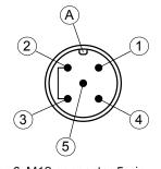
Fig. 6: M12 connector 5-pin
