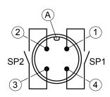
Fig. 7: M12 connector 4-pin
