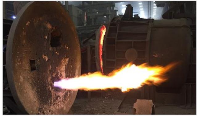
Ladle Heating Systems
