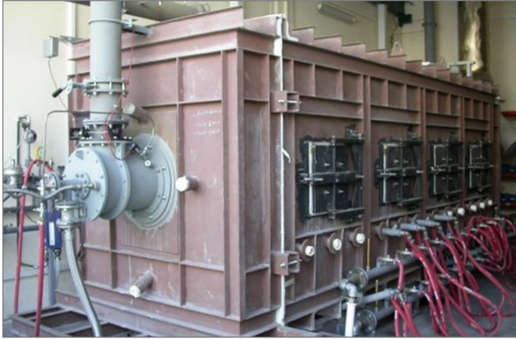
A.T. BURNER TEST FURNACE
